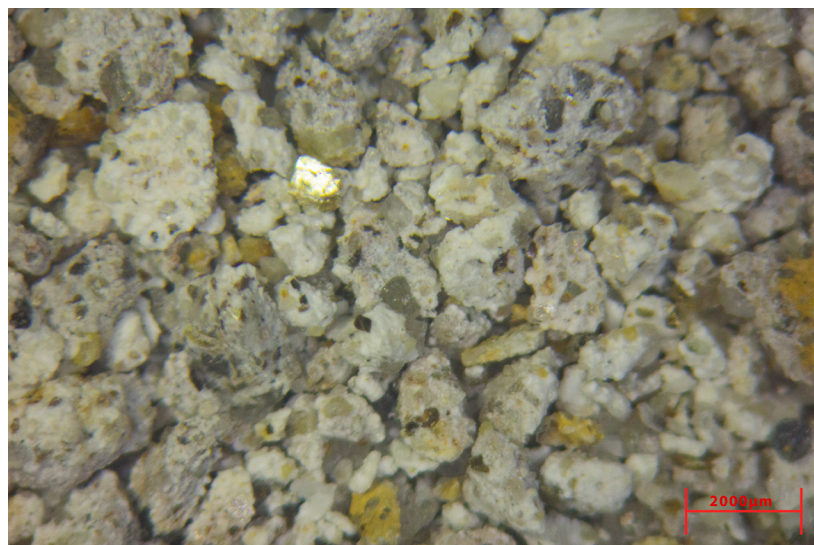
Photomicrograph of the extracted aggregate before sieving, note the abundant undigested binder clumps (incident daylight-balanced light, 10x magnification).
