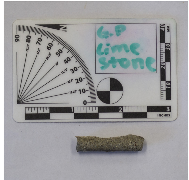
Photograph of the weathered face of the bulk sample before digestion (fluorescent light, color corrected).
