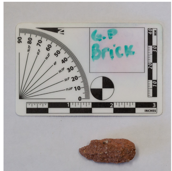
Photograph of the weathered face of the bulk sample before digestion (fluorescent light, color corrected).
